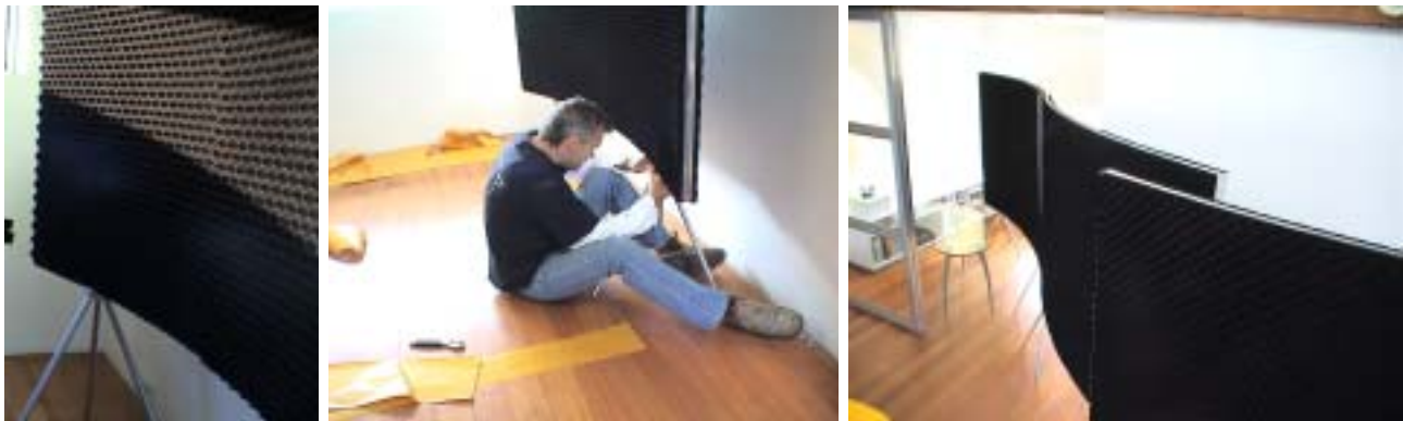
Above: Completed acoustic foam partition screen showing the surface, David Poulton completing assembly of the legs, assembled screens arranged as partition wall
