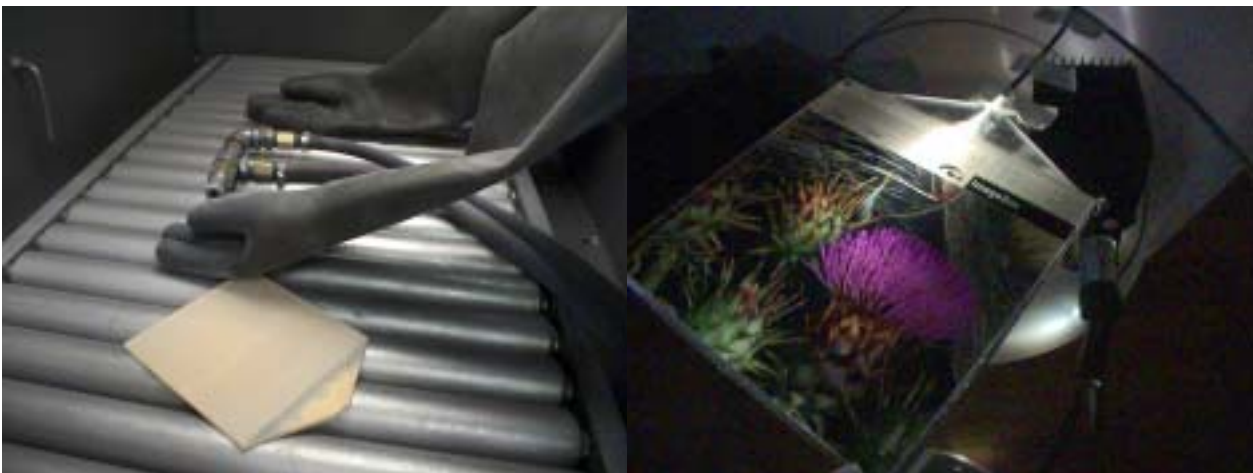
Above: The sandblasting booth setup used to test the sandblasting options for the acrylic light guides, The first lighting test being conducted on a sample light guide sandwich
