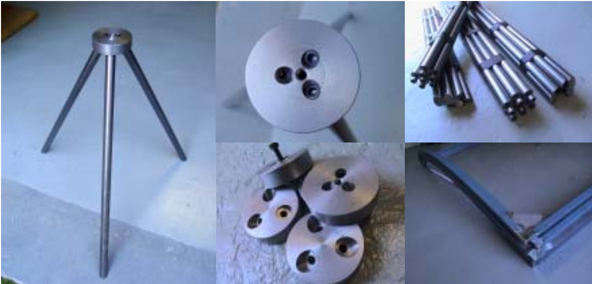
Above: Images of the modular machined tripod leg base system developed to support the partition screens used in conjunction with the Screen Lounge pods.
