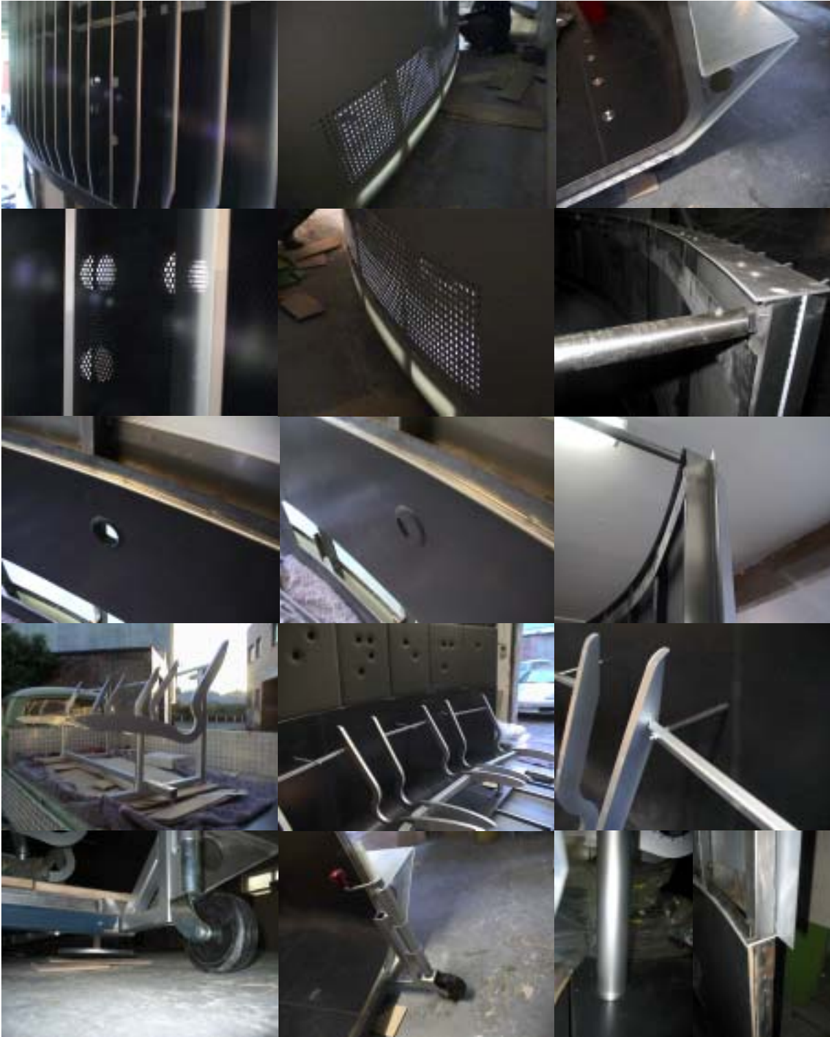
Above from top left: louvre wall fitted with interior panels, external aluminium skin with venting behind the Mantle Boot for the computers, end aluminium trim with internal lighting stainless steel cover plates, louvre wall fitted with interior panels, external aluminium skin with venting, top rail, cable port for the plasma monitor, top rail and stainless steel end trim, painted seating chassis, seating chassis installed, detail of seat chassis anchor, trolley wheels in place, seat chassis anchor, extruded skin detail
