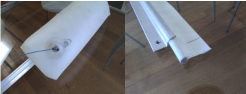
Images of the polyurethane test inflatable and the rope track/track lock system components to secure the inflatable ceiling to the Screen Lounge pod walls.
