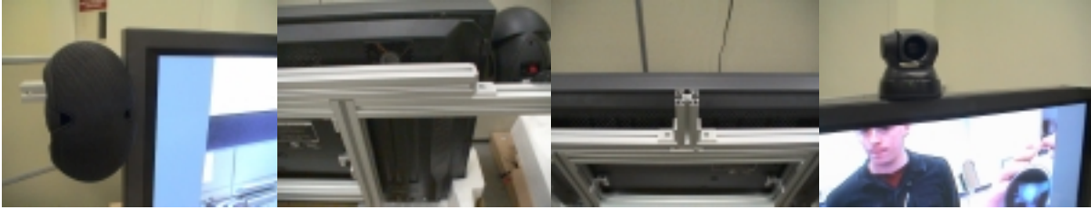
Images of the AME system bracket developed by Matthew Mulcahy of ACMI to hold the speakers and video camera to the plasma monitor
