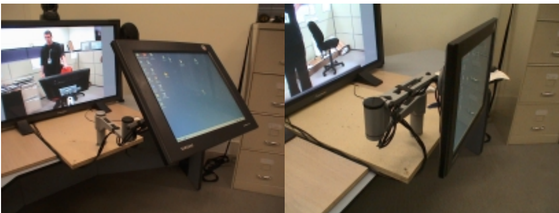
Images of the prototype installation set up by Matthew Mulcahy at ACMI showing the plasma monitor and the LCD touch screen mounted on the Spacedec arm. Right shows the stowed position of the Spacedec arm [within the Mantle Boot].
