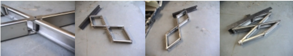
Images of the Scissor Arm prototype with the increased wall thickness and additional returns to achieve a very high level of stiffness
