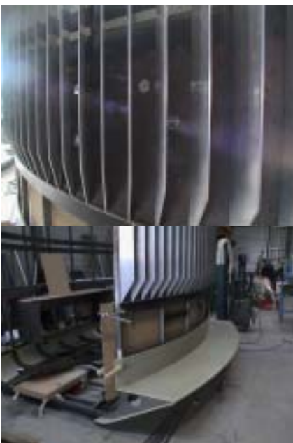
Left and below: Fitting the aluminium skin to the frame. Details of the internal panel tab system, aluminium skin rear Mantle Boot vent and the composite louvre wall/mesh and peephole membrane construction.
