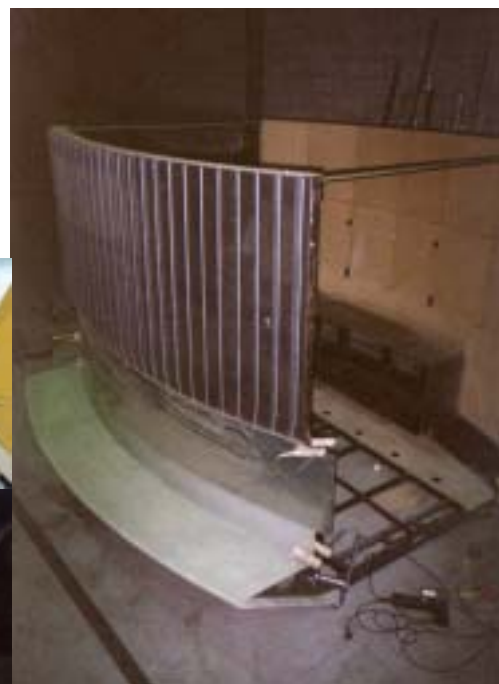
Left and below: Fitting the aluminium skin to the frame. Details of the internal panel tab system, aluminium skin rear Mantle Boot vent and the composite louvre wall/mesh and peephole membrane construction.
