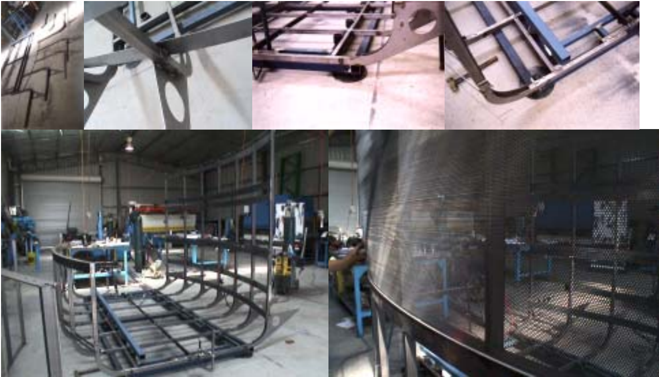
Documentation of the fabrication of 01 production Screen Lounge pod frame. Above: main frame assembly and fitting the mesh skin located behind the louvre wall.
