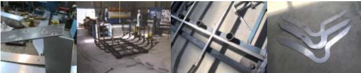
Documentation of the fabrication of 01 production Screen Lounge pod frame. Above: main frame assembly and fitting the mesh skin located behind the louvre wall.
