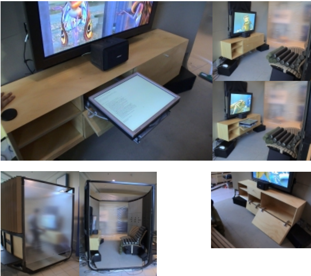
Clockwise from top left: Mantle Piece control console with touch screen fully extended, Mantle Piece control console with touch screen fully retracted, Mantle Piece control console with touch screen fully extended, Mantle Piece control console with touch screen fully retracted and the technology boot open. Screen Lounge Pod interior with mocked up end wall to emulate the presence of a translucent end wall, Screen Lounge Pod with mocked up end wall to emulate the presence of a translucent end wall seen from outside.
