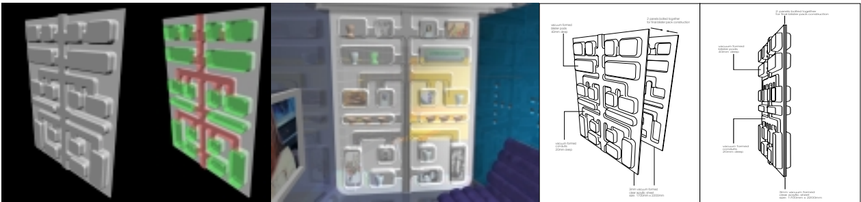
Images of two seater Screen Lounge Pod in translucent fibreglass and matt etched mirror aluminium skin and black acoustic partition.
